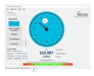
Perform mounting verification & rotation direction selection before calibration to ensure optimal performance.
