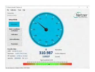
In case the reading data (blue dots) are not evenly distributed on a thin circle, you may experience "noise" in your installation (check shaft/stator grounding).
