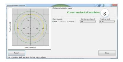
**(h)** If the SW indicates "Incorrect Mounting," correct the mechanical position of the rotor, as presented in paragraph 5.1 - "Encoder stator / Rotor relative position".
