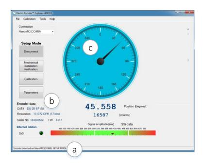
Perform mounting verification & rotation direction selection before calibration to ensure optimal performance. It is also recommended to observe the installation at the [Tools - Signal Analyzer] window.
