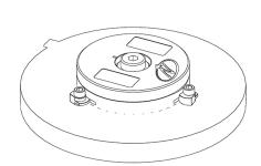
The encoder rotor (2) is attached to the host shaft (d) by pressing it against a dedicated shoulder (a), while using screw and a washer, or a circular spring and a washer, at the top of the shoulder to maintain downward pressure. Recommended torque of 0.3 Nm with M3 screw.
