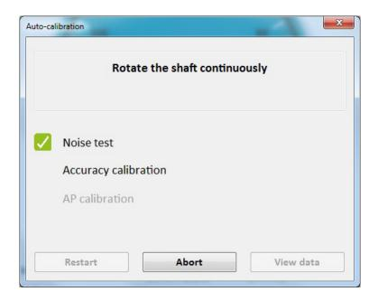
Once the noise test is successful, start rotating the shaft continuously until the auto-calibration process ends.
