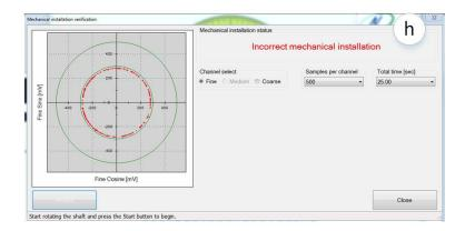
The Signal Analyzer window [Tools - Signal Analyzer] can also be used to verify the signals are good for an installed encoder.
