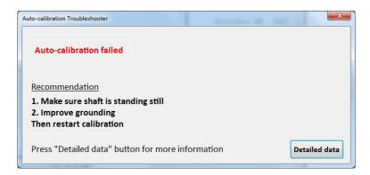
Pressing the "Detailed data" button, will display detailed information regarding the failure.
