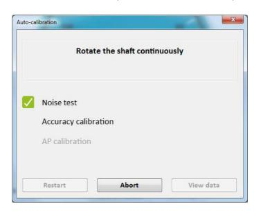
Once the noise test is successful, start rotating the shaft continuously until the auto-calibration process finishes.
