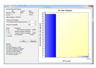
In case the reading data (blue dots) are not evenly distributed on a thin circle, you may experience "noise" in your installation (check shaft/stator grounding).
