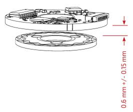
Note: The rotor adaptor should be made from a non metal material.
